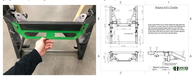
**Rear frame** may be altered to accept leaf, coil spring, or coil-over. . No fiberglass graphite or exotic springs permitted. Must be of magnetic steel be a maximum retail cost of \$120.00 ea "leaf spring max cost is \$175.00 ea" No fiber glass lift bars. No torsion bars in rear. **The rear center link may be a solid link or mounted in rubber bushings.** No spring third links or trailing arms allowed.
